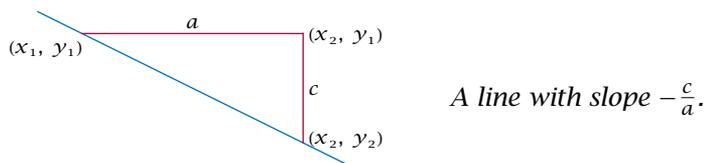
In the figure above,  $a$  is the length of the horizontal line segment and  $c$  is the length of the vertical line segment. Of course  $a$  and  $c$  are positive numbers, because lengths are positive. In terms of the coordinates as shown in the figure above, we have  $a = x_2 - x_1$  and  $c = y_1 - y_2$ . The slope of this line equals  $(y_2 - y_1)/(x_2 - x_1)$ , which equals  $-c/a$ .
