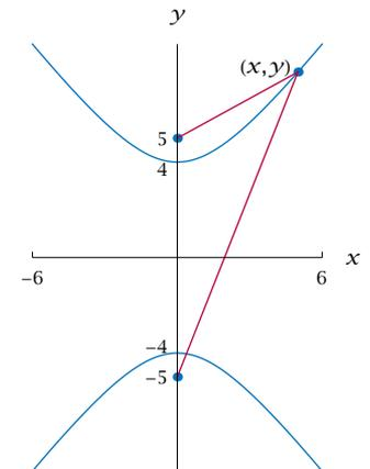
For every point  $(x, y)$  on the hyperbola  $\frac{y^2}{16} - \frac{x^2}{9} = 1$ , the difference of the lengths of the two red line segments equals 8.
