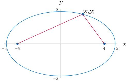
For every point  $(x, y)$  on the ellipse  $\frac{x^2}{25} + \frac{y^2}{9} = 1$ , the sum of the lengths of the two red line segments equals 10.
