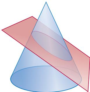
The ancient Greeks discovered that the intersection of a cone and an appropriately positioned plane is an ellipse.
