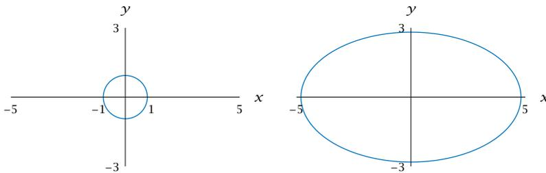
Stretching horizontally by a factor of 5 and vertically by a factor of 3 transforms the circle on the left into the ellipse on the right.
