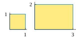
More generally, suppose  $c$ ,  $d$  are positive numbers, and consider the transformation that stretches horizontally by a factor of  $c$  and stretches vertically by a factor of  $d$ . This transformation changes a square whose sides have length 1 into a rectangle with base  $c$  and height  $d$ , as shown here. Thus the area has been increased by a factor of  $cd$ .
